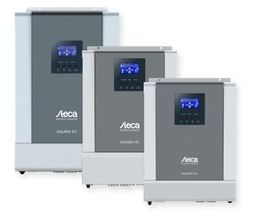
The Steca Solarix PLI is the first product from Steca Elektronik to offer an all-in-one package. It allows users to supply consumers with 230 V AC power, charges the battery with an integrated MPPT charge controller, and at the same time permits connection to a generator or an available electricity grid. Everything in a single device.
