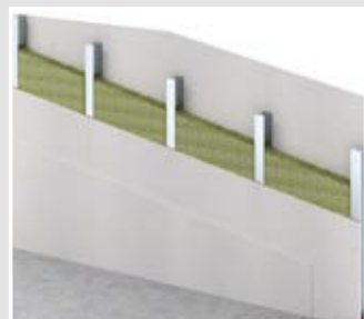
Installation of F90 metal stud walling in compliance with DIN 4102, Part 4
