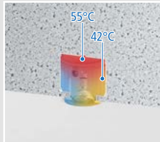
Temperature profile HV halogen luminaire max. 75 W (230V)
