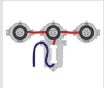
Schematic diagram of group switching with a operating device.
