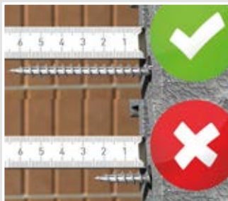
The dowel screw must protrude from the basic element by at least 40 mm.
