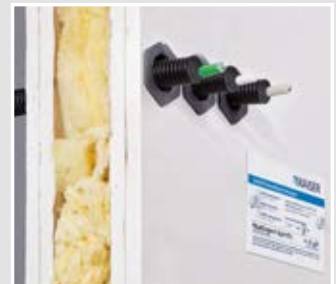
The conduit sealings can be arranged vertically or horizontally to form a group with a centre distance of 50 mm.
