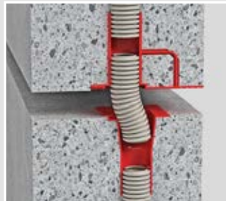
Compensation in transverse direction \pm 10 mm.
