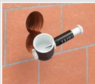
The flush-mounting fire-protection box provides 6 entry options for conduits up to M25 and cables up to \varnothing 11.5 mm
