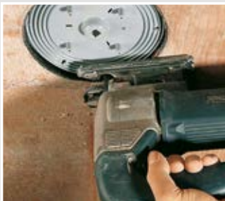
Open front part using a fretsaw.
